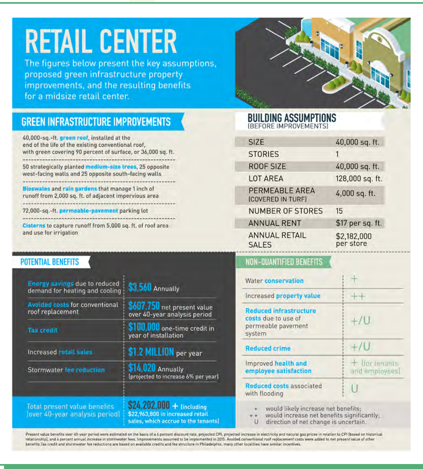
Figure 4. Application of benefits transfer to estimate benefits of GSI installation for hypothetical retail center (2013 USD).
